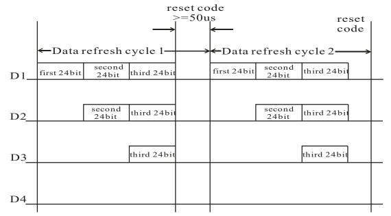
Note: The data of D1 is send by MCU, and D2, D3, D4 through pixel internal reshaping amplification to transmit.
